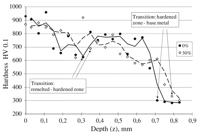
Fig. 4 Microhardness measurements cross the modified layer at different overlapping degrees of the remelted traces
